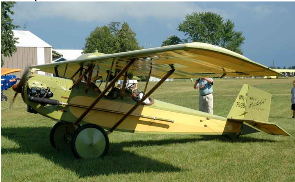
Another view of Douwe's Pietenpol. Notice the wooden lift struts and cabane struts.
