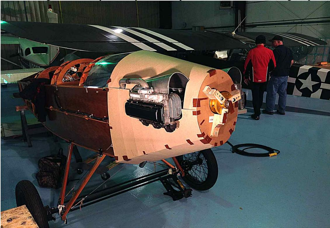
Today (3/28/13) was a milestone as I cut the first metal for the engine cowl. Here is what it looks like with the nose bowl in place and the top half of the cowl cut and clecoed in place.
